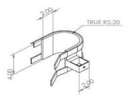
Figure 1 Schematic design for the thigh brace
